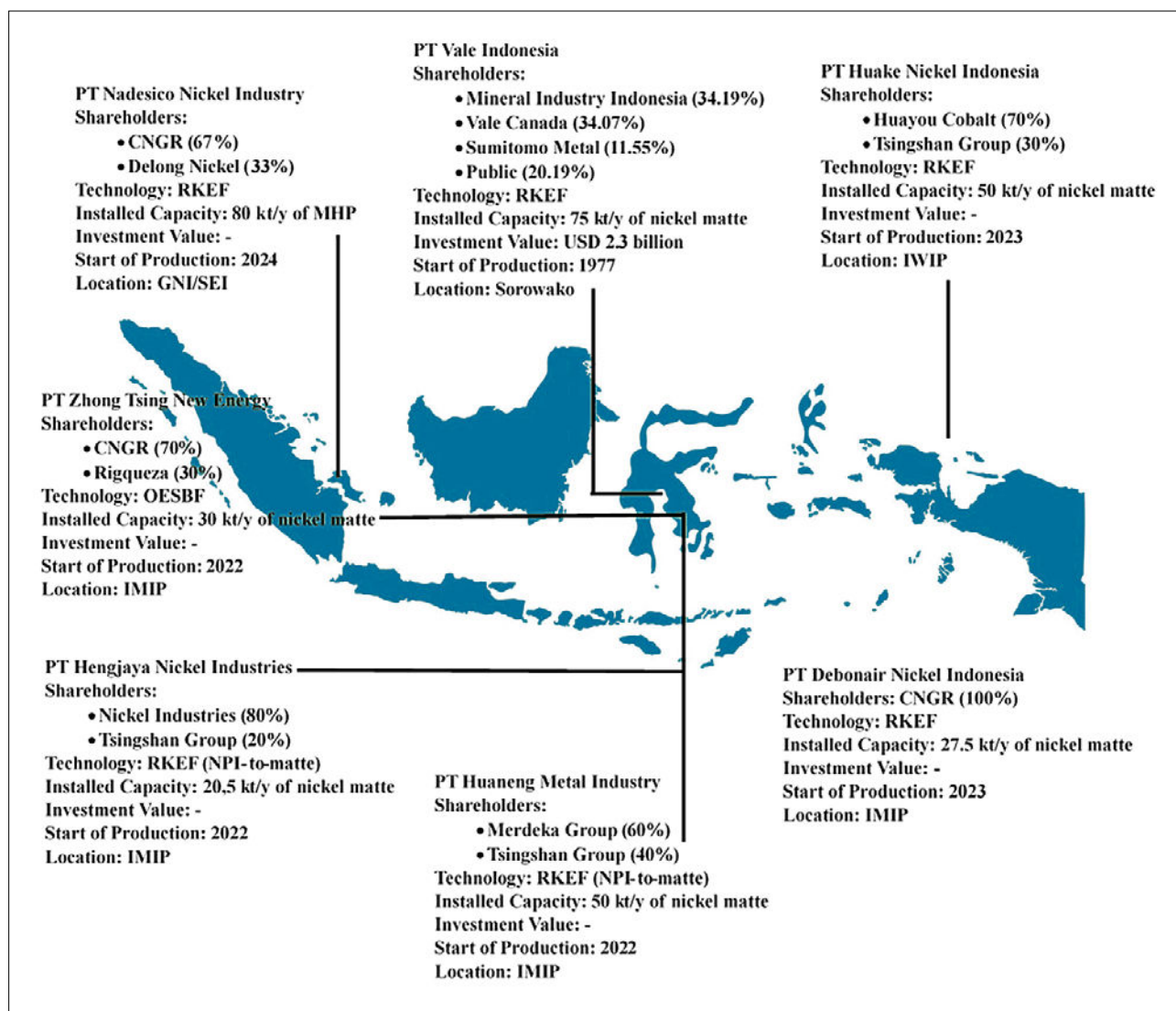
Figure 11. Nickel matte facilities operating in Indonesia
